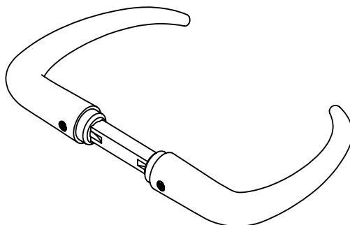
**Spare parts/** 14970102019 - Grub screw M5x8,3mm
